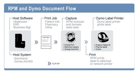
Document Flow Diagram for RPM and Dymo Label Printers: Host system sends document or print data to RPM via TCP/IP. RPM massages the label data (margins, fonts, orientation, etc.) to prepare it for printing. RPM sends the reformatted label data to Dymo label printers for local or network printing.
